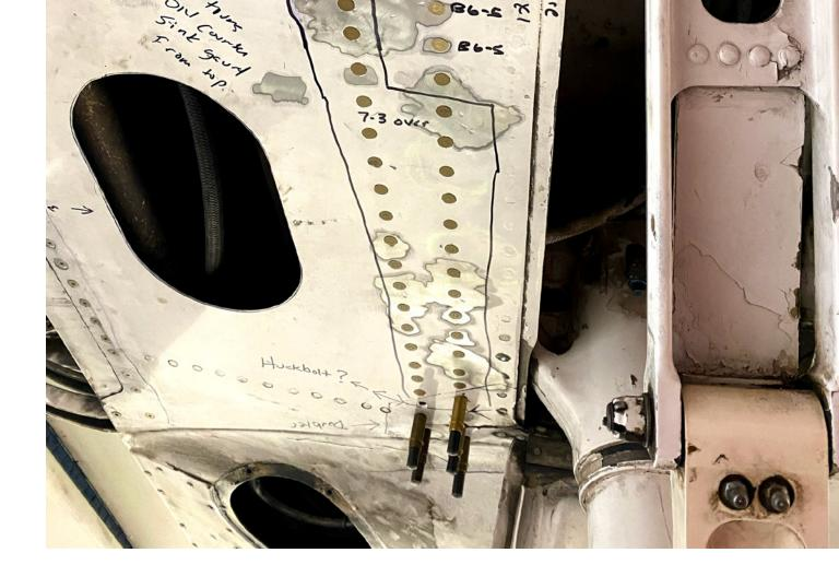
served the smaller diameter countersunk head of the OEM fastener had almost pulled through. They would require countersinking to a bigger head Hi-Lok with the same shank diameter.
